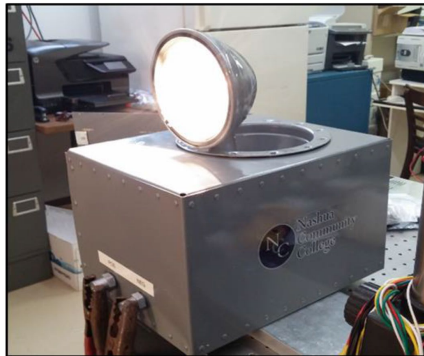
Figure 4. Prototype PAR46UVLED landing light operating in a test fixture
